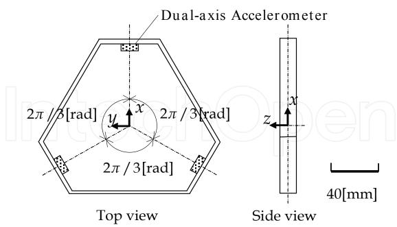
Fig. 4. Outline drawing of a prototype 6-DOF accelerometer
