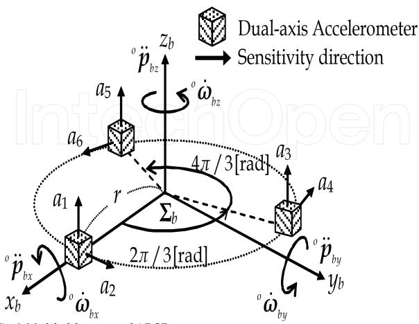
Fig. 2. Model of the proposed 6-DOF measurement system
