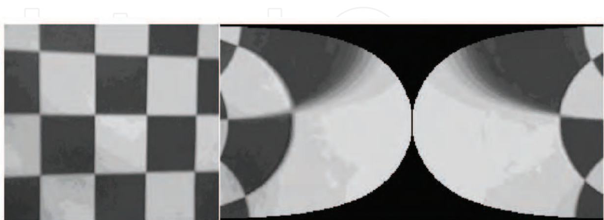
Fig. 7. Collicular mapping according to equation (3) with interpolated uniform resolution. Left: the image acquired by the camera; Right: the two halves of the image mapped with the collicular geometry expressed by equation (3).
