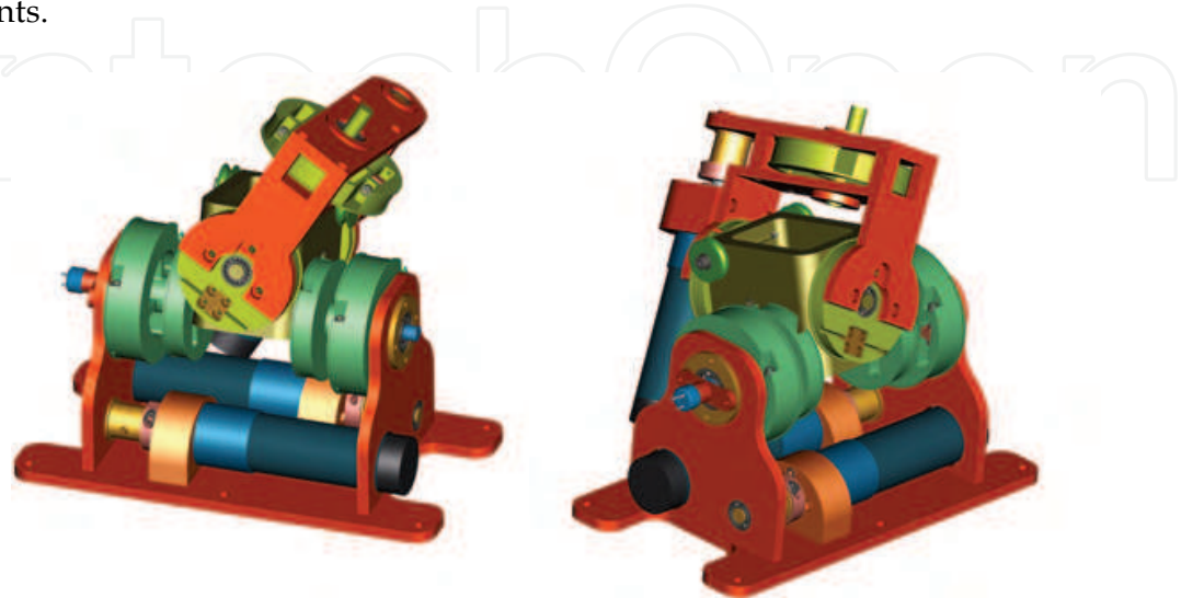
Fig. 1. CAD captures of the differential drive to be used as the robot waist.
