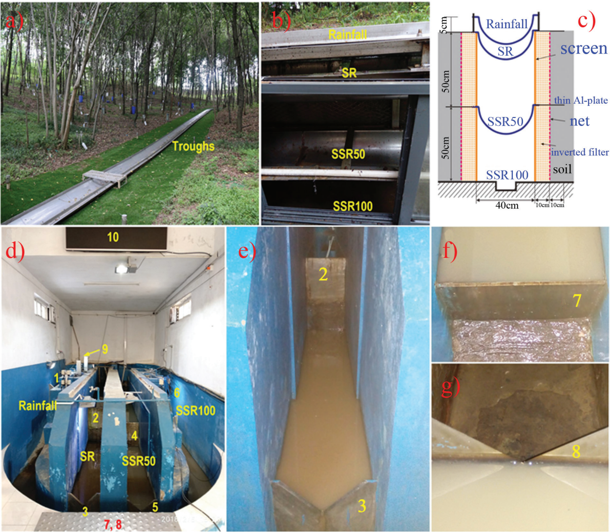
Figure 5. Instrumentation for runoff measurement in Nandadish: (a) Main trench with troughs (not shown), (b) the branch trench with four troughs (previously Figure 13c ), (c) schematic figure illustrating various troughs, (d) discharge measurement structures for different runoff components from troughs 1 for rainfall; 2 and 3 for surface runoff; 4 and 5 for interflow (50 cm below the soil surface); 6 for interflow and groundwater flow (down to bedrock); 7 and 8 for total runoff (weirs are shown (f) and (g)). 1, 3, 5, 6, and 8 are 90° V-notch weir; 2, 4 and 7 are the full width rectangular weirs; 9 is the probe-type water level gauge; 10 is a video for monitoring the runoff processed, (e) combination of a 90° V-notch weir and a full width rectangular weir for SR, SSR50, and the total runoff, (f) the full width rectangular weir for total runoff, (g) the 90° V-notch weir for total runoff.
