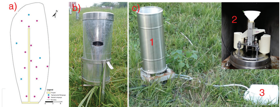
Figure 14. Instrumentation for precipitation measurement in Hydrohill: (a) locations of 12 standard rain gauges and 5 tipping bucket rain gauges; (b) a standard rain gauge; (c) a tipping-bucket rain gauge. 1-external structure, 2-internal structure, 3-a plastic pot used to collect total precipitation of each event.
