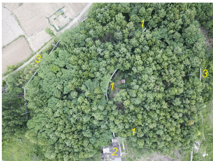
Figure 3. The bird’s eye view of the forested Nandadish watershed taken at May 2018. 1-trench with layered troughs; 2-block divider; 3-house for discharge measuring structures.
