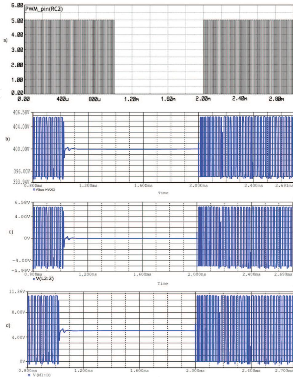
**Figure 13.** Simulation results at the transmitter: (a) PIC 16f876A microcontroller modulated signal, (b) 400V HVDC bus signal, (c) Signal curve at transformer inductance Lp2 also katot diode, (d) Amplified signal at drain MOSFET.
