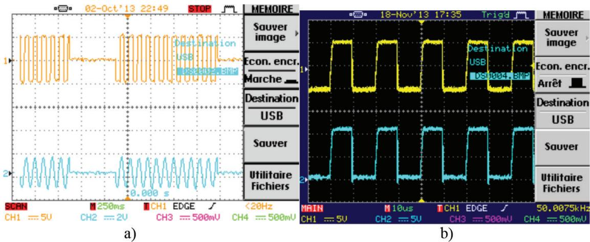
**Figure 16.** Curves obtained at the oscilloscope: (a) yellow signal curve transmitted on the line and blue output signal curve on the receiver filtering stage; (b) young Lp2 inductance signal and emitter drain signal M1.
