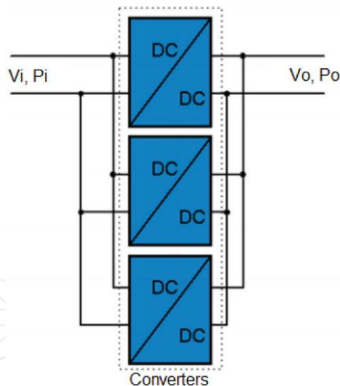
**Figure 3.** Connecting converters in parallel.
