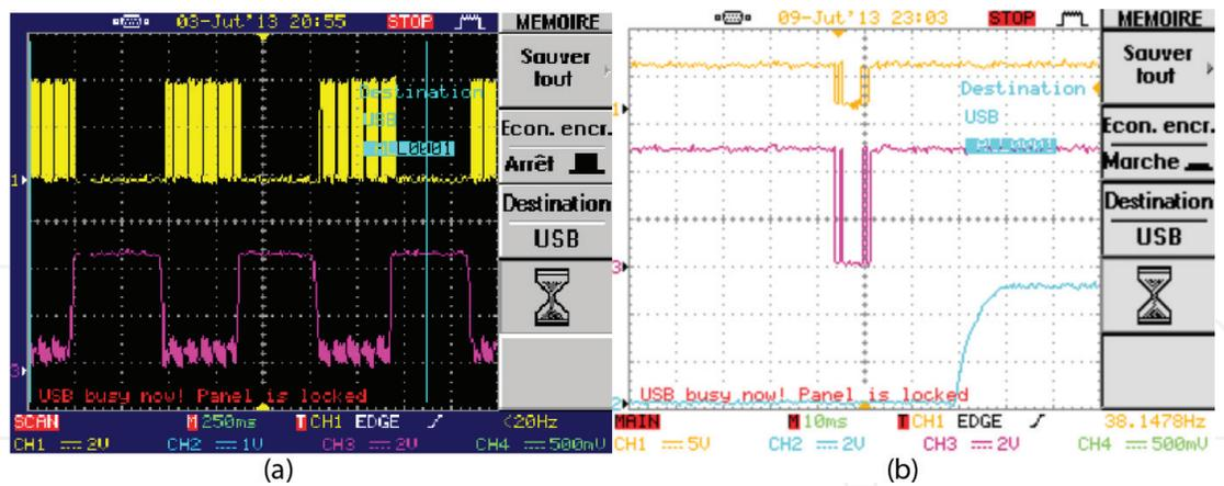
**Figure 15.** (a) Oscilloscope curves in model tests: yellow modulated signal with microcontroller of the transmitter and violet output signal of the receiver; (b) RS232 low data signal, positive logic: yellow TX/RC6 signal and purple RX/RC7 microcontroller signal.
