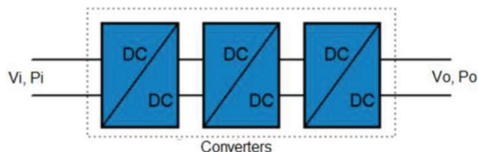
**Figure 4.** Connection of converters in cascade.
