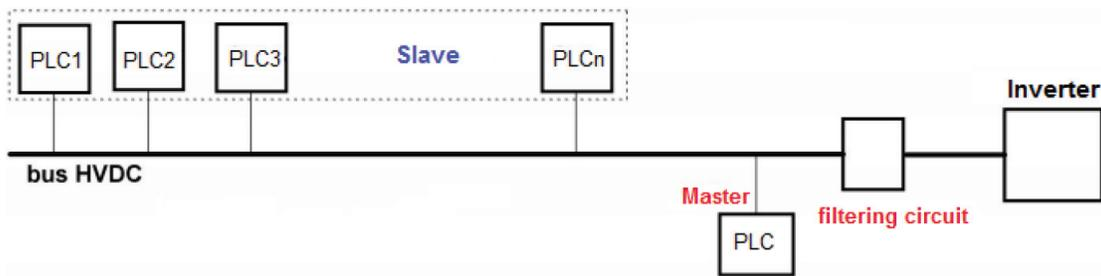
Figure 17. Diagram of master-slave HVDC PLC systems.
