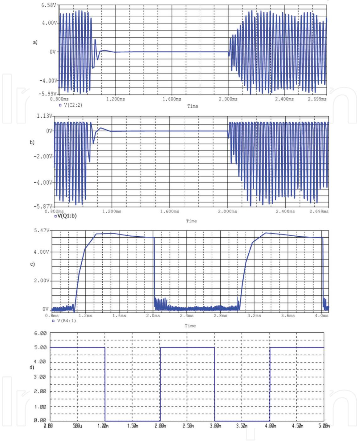
**Figure 14.** Simulation results at the receiver: (a) signal curve at the low band filtering circuit R1, C1, (b) input signal at the base of transistor Q1, (c) amplified signal at the collector of transistor Q1, (d) output signal A/D conversion.
