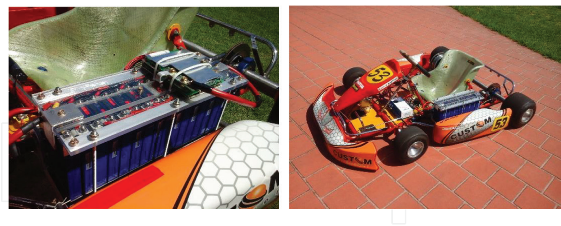
Figure 9. 48 V Lithium-ion battery pack with BMS and the prototype electric kart.
