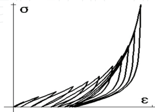
Figure 32. Modeling of ferroelastics: small hysteresis loops.
