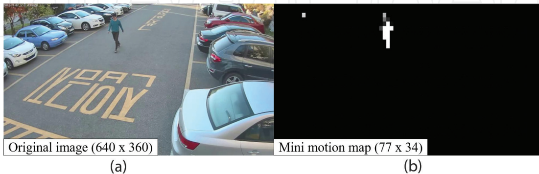
Figure 3. Mini motion map for reducing the unnecessary computation in the HOG-based human detector: (a) original image with a size of 640 \times 360 and (b) mini motion map with a size of 77 \times 34 , which was calculated from the GMM-based motion detection.
