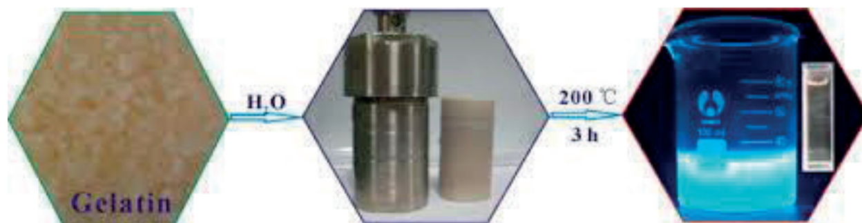
Figure 6. Synthesis of blue emissive carbon quantum dots from gelatin via hydrothermal carbonization process (reproduced with permission from [7]).
