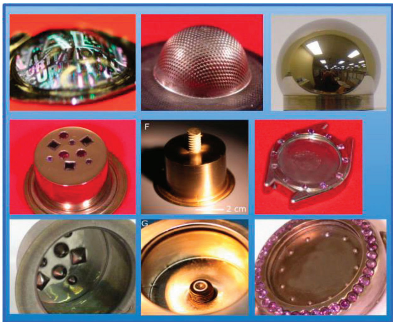
Figure 3. These shapes were previously unachievable with any other metal processing method that can be fabricated by blow molding [46].
