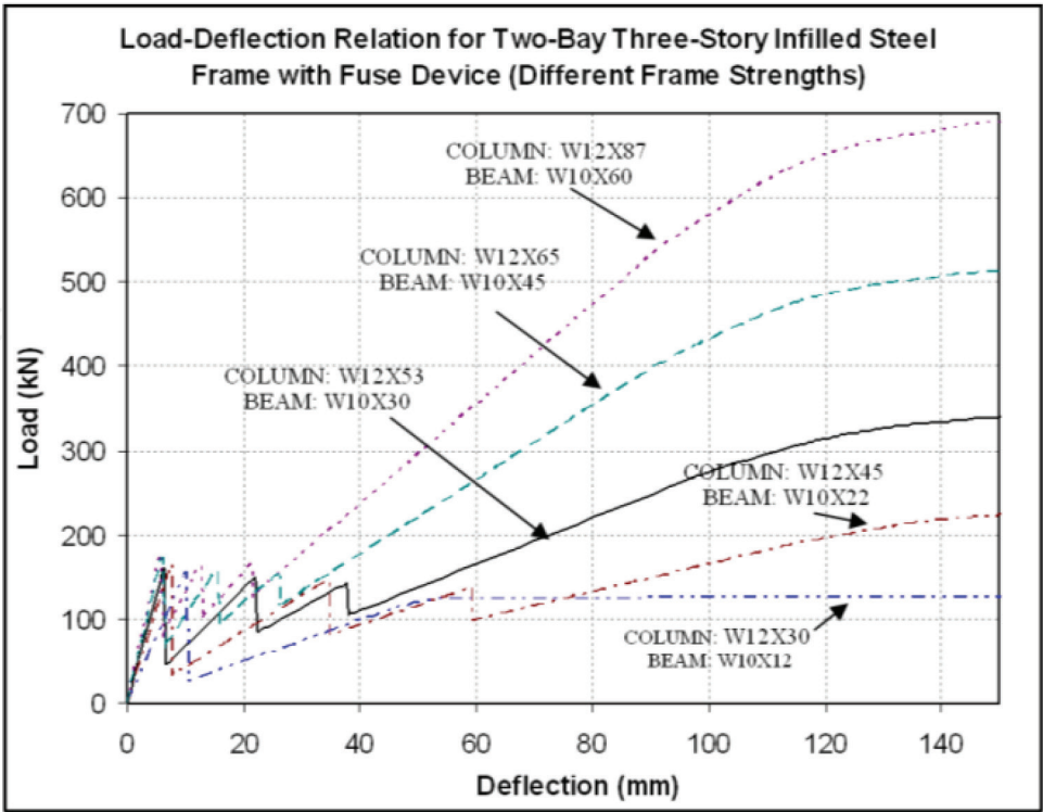
Figure 30. Load-deflection relation for two-bay, three-story infilled steel frame with fuse system with different frame Strengths [53].
