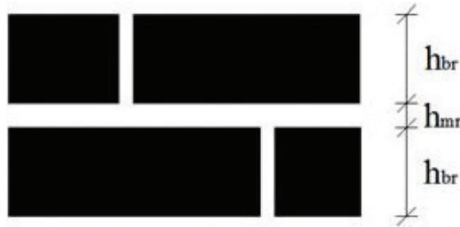
**Figure 2.** Assumption for the discontinuity surface between two units along the thickness of the mortar resulting failure of the wall [13].
