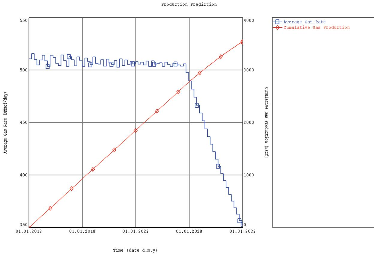
Figure 11. Production profile of the 50 production wells.
