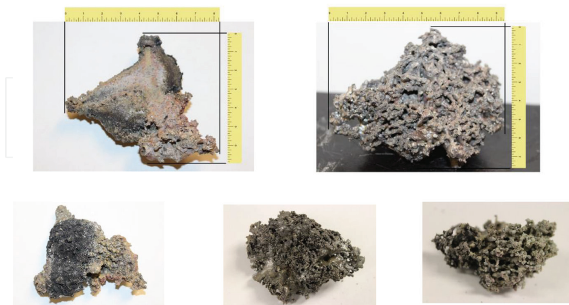
Figure 7. Clinkering during gasification of composite pellet of fiber and plastic (unit: cm) [25].
