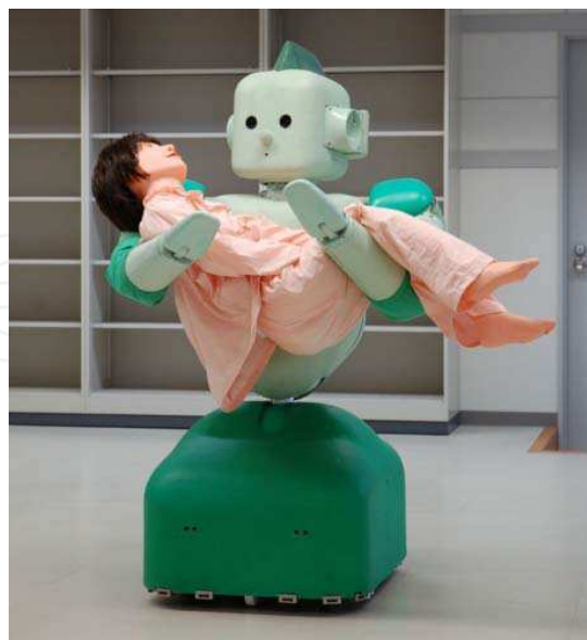
Fig. 1. RI-MAN with tactile sensors for physical human-robot interaction research
