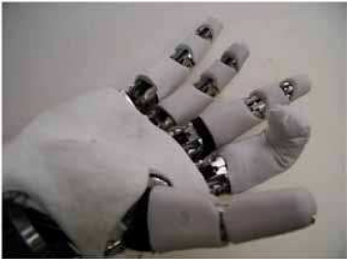
Fig. 5. Placement of the pressure transducers in the Robonaut hand (Martin et al., 2004).
