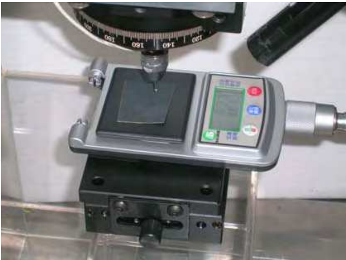
Fig. 17. The probe touches down the electronic scales.
