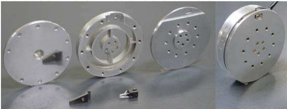
Fig. 12. Optical torque sensor with ring-shaped flexure
