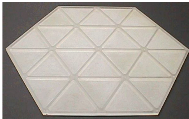
Figure 17. 305 mm wide mirror made from 5.3 mm thick ultra-low expansion glass with pockets milled to 3.6 mm deep.
