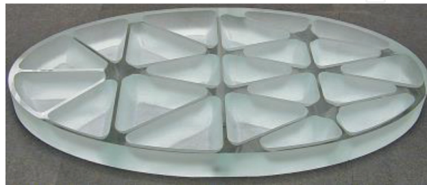
Figure 16. 250 mm (major axis) elliptical mirror with pockets milled to 9.5 mm deep.
