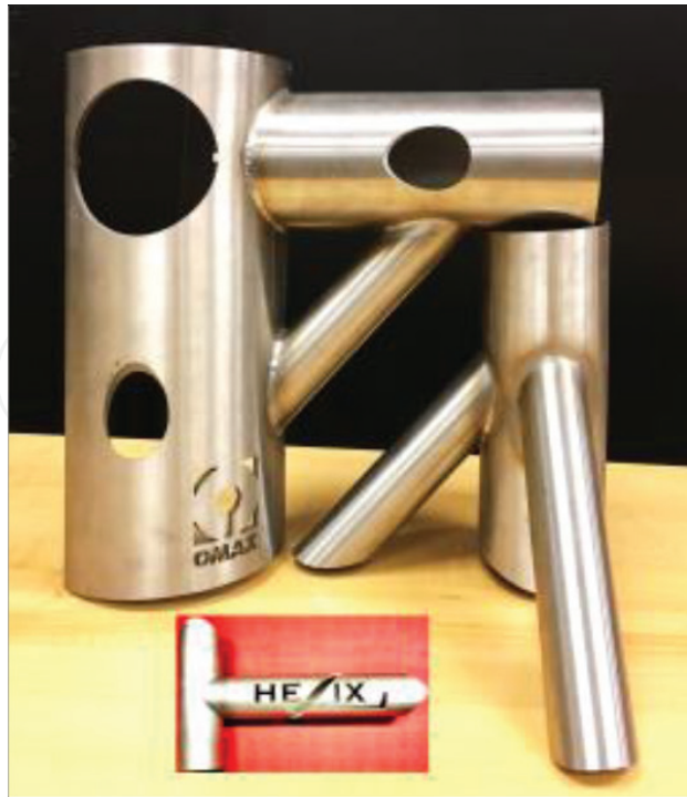
Figure 14. AWJ-cut “Fish mouth” weld joints.
