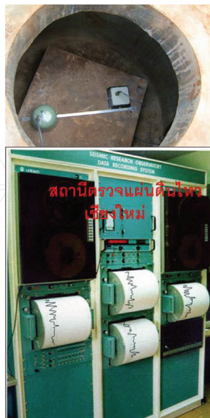
Figure 3. Installation of velocity sensor and accelerometer at CMMT seismic station (Thai Meteorological Department) [5].
