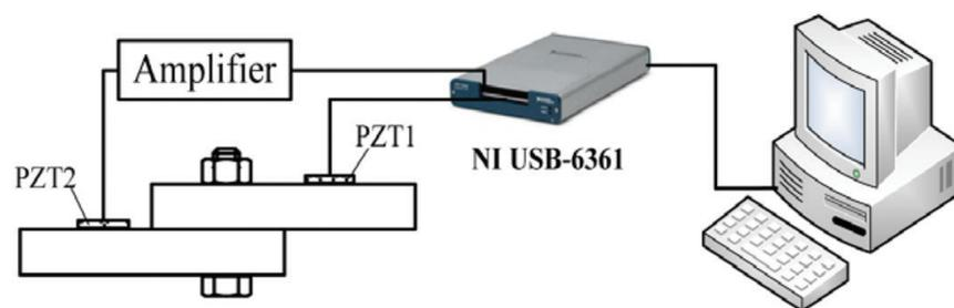
**Figure 5.** Schematic of the bolt joint monitoring system [26].
