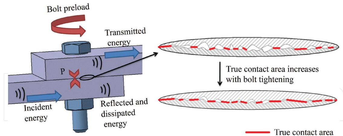
Figure 1. Guided wave transmitted across a bolted joint.
