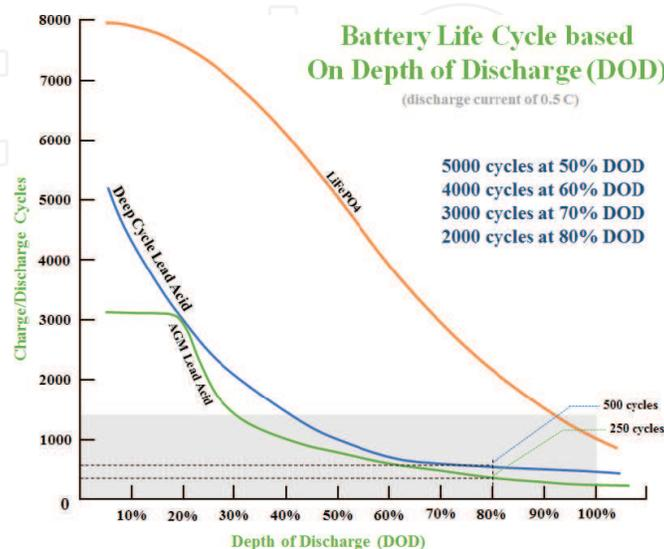
**Figure 6.** Relationship between DoD and charge/discharge cycles (life cycles) modified from [49].
