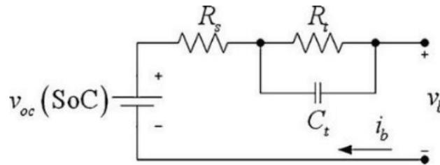
Figure 9. A generalized ECM for lithium batteries.
