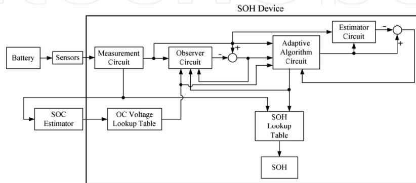
Figure 10. A flowchart describes how SoH functions.
