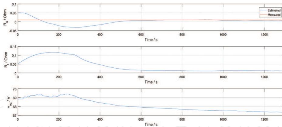
Figure 11. Comparison of estimated and measured internal resistances (1st,  $R_s$ ; 2nd,  $R_t$ ) and VoC (voltage of open circuit) in test case.
