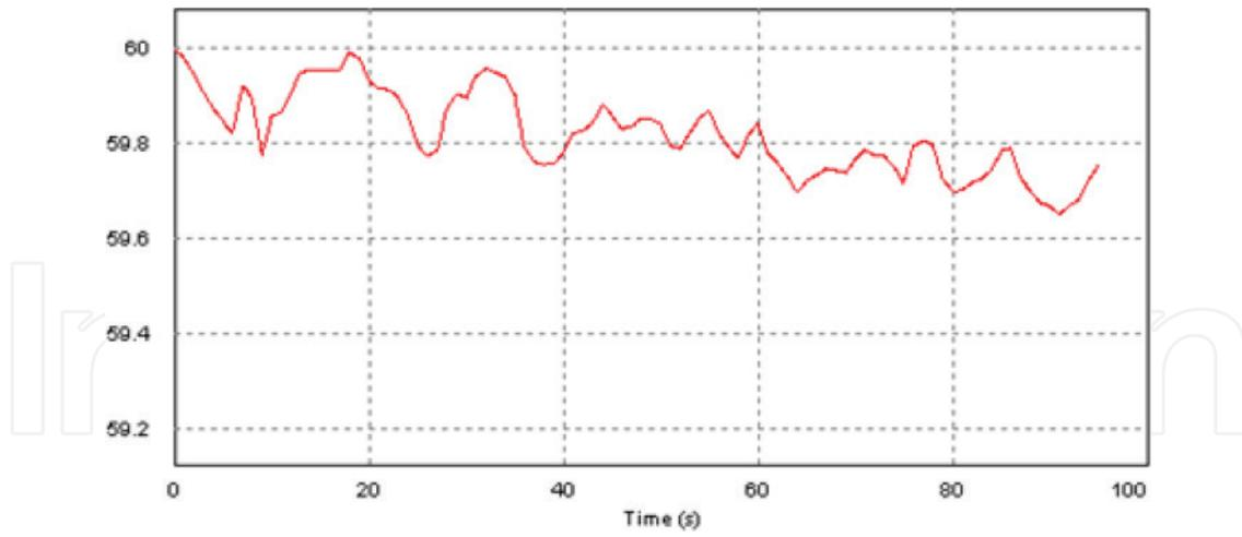
Figure 14. Voltage drop in simulation of 60 V single RLIB pack.
