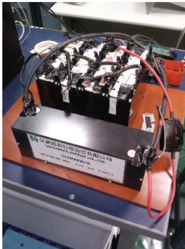
**Figure 12.** Implementation of RLIB with EMS and auxiliary physical battery (left: EMU; Central: LiFePO<sub>4</sub> LIB pack; and right: auxiliary physical battery).
