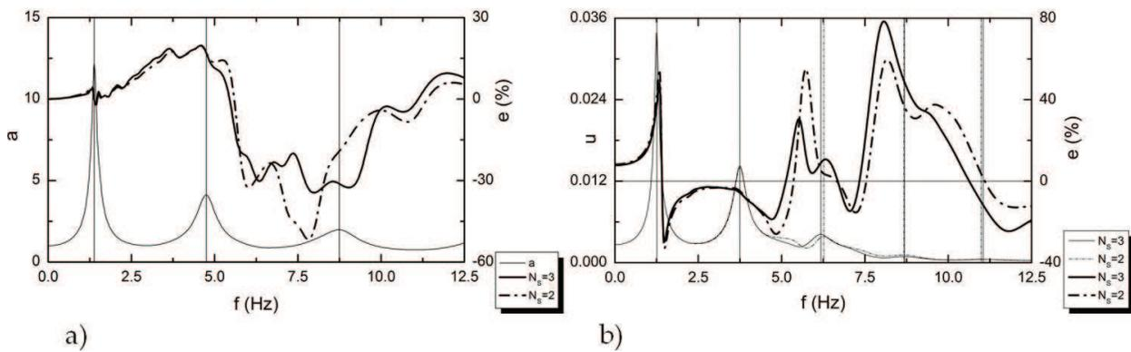
**Figure 15.** Interaction between surface structure and underground structure in terms of harmonic response spectra and influence coefficient  $e$  for different number of span of underground structure under S waves producing motions on the Y axis ( $d = 0.5$ ), a) the impact on surface structure, b) the impact on underground structure.
