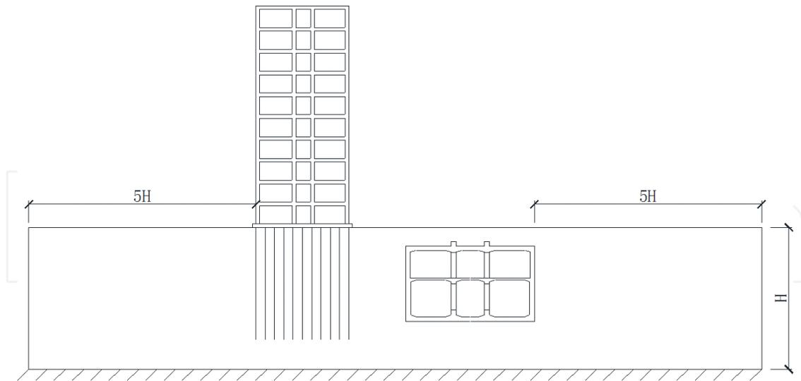
**Figure 4.** Arrangement of structures and soil (AR1).
