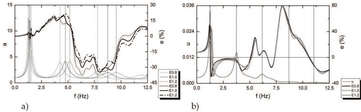
**Figure 11.** Interaction between surface structure and underground structure, arranged according to AR1, in terms of harmonic response spectra and influence coefficient  $e$  for different stiffness of surface structure under S waves producing motions on the Y (frame structure,  $d = 0.5$ ), a) the impact on surface structure, b) the impact on underground structure.
