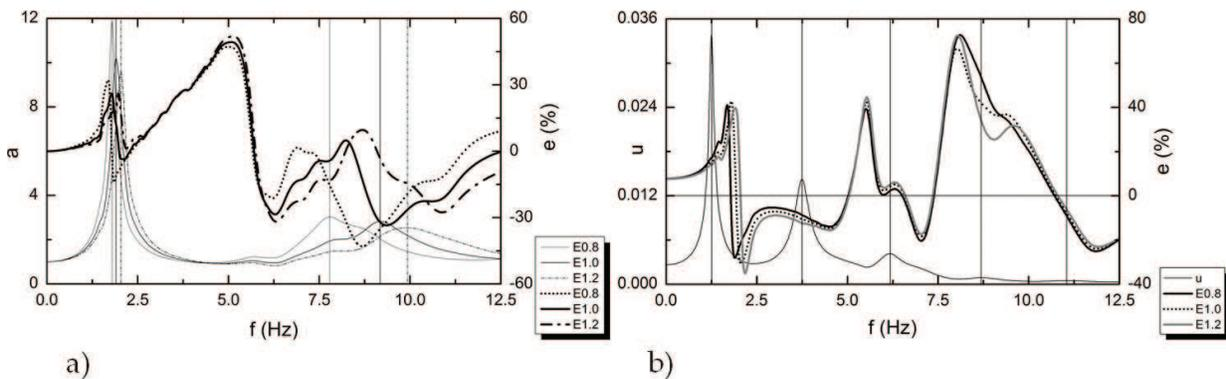
**Figure 12.** Interaction between surface structure and underground structure, arranged according to AR1, in terms of harmonic response spectra and influence coefficient  $e$  for different stiffness of surface structure under S waves producing motions on the Y axis (frame-shear wall structure,  $d = 0.5$ ), a) the impact on surface structure, b) the impact on underground structure.
