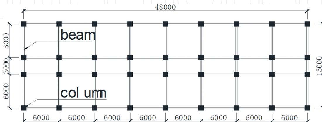
**Figure 1.** Typical plan of surface structure (unit: Mm).
