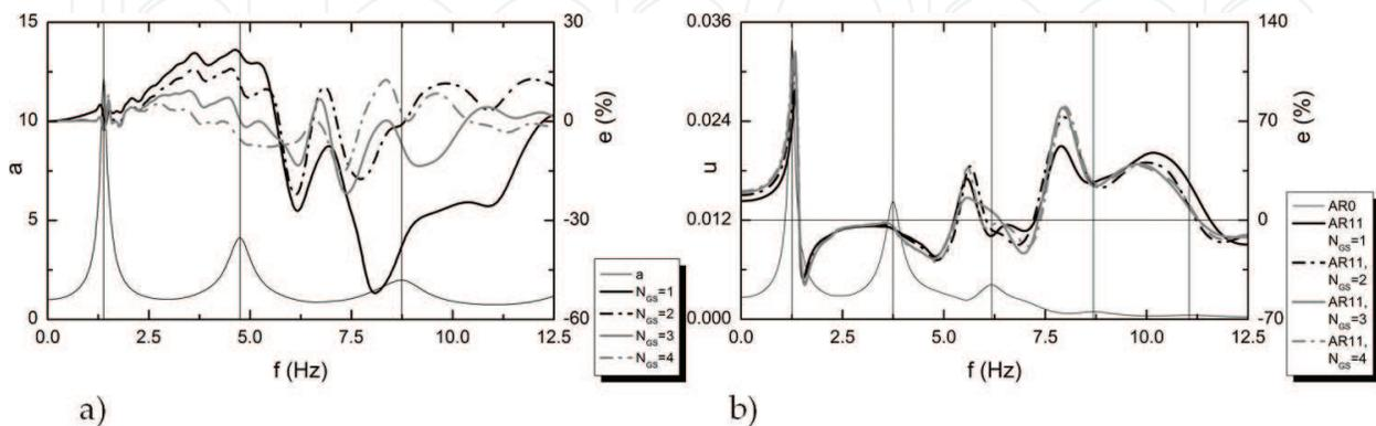
**Figure 16.** Interaction between surface structure and underground structure in terms of harmonic response spectra and influence coefficient  $e$  for different numbers of surface structures under S waves producing motions on the Y axis ( $d = 0.1$ ), a) the impact on surface structure, b) the impact on underground structure.
