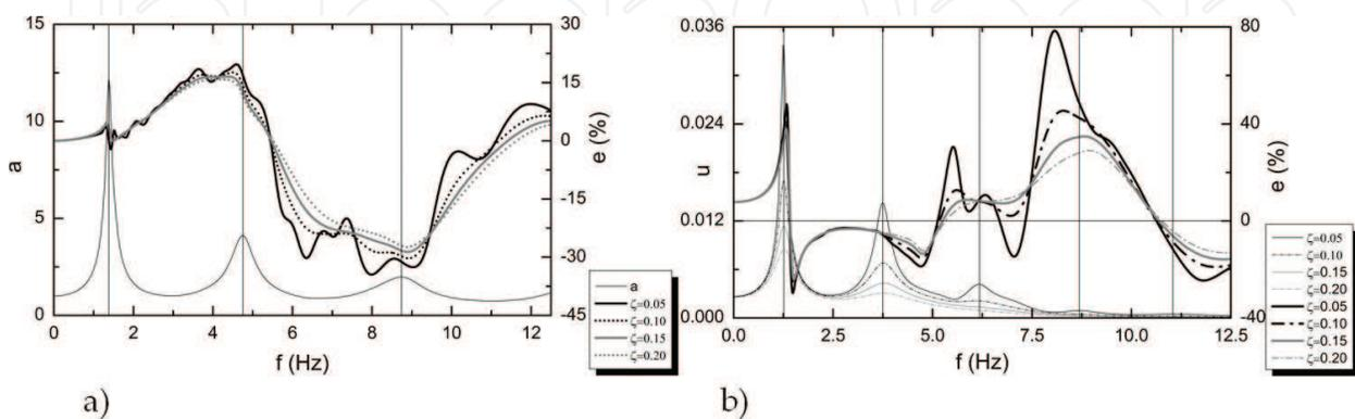
**Figure 8.** Interaction between surface structure and underground structure, arranged according to AR1, in terms of harmonic response spectra and influence coefficient  $e$  for different soil damping under S waves producing motions on the Y axis ( $d = 0.5$ ), a) the impact on surface structure, b) the impact on underground structure.
