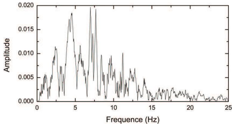
**Figure 19.** Fourier spectrum of seismic wave (GGP-100).
