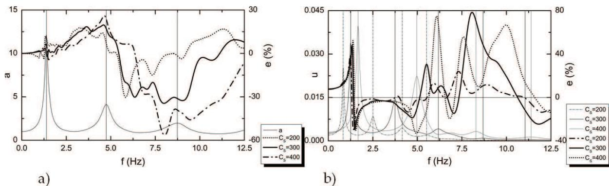
**Figure 9.** Interaction between surface structure and underground structure, arranged according to AR1, in terms of harmonic response spectra and influence coefficient  $e$  for different shear wave velocity of soil under S waves producing motions on the Y axis ( $d = 0.5$ ), a) the impact on surface structure, b) the impact on underground structure.
