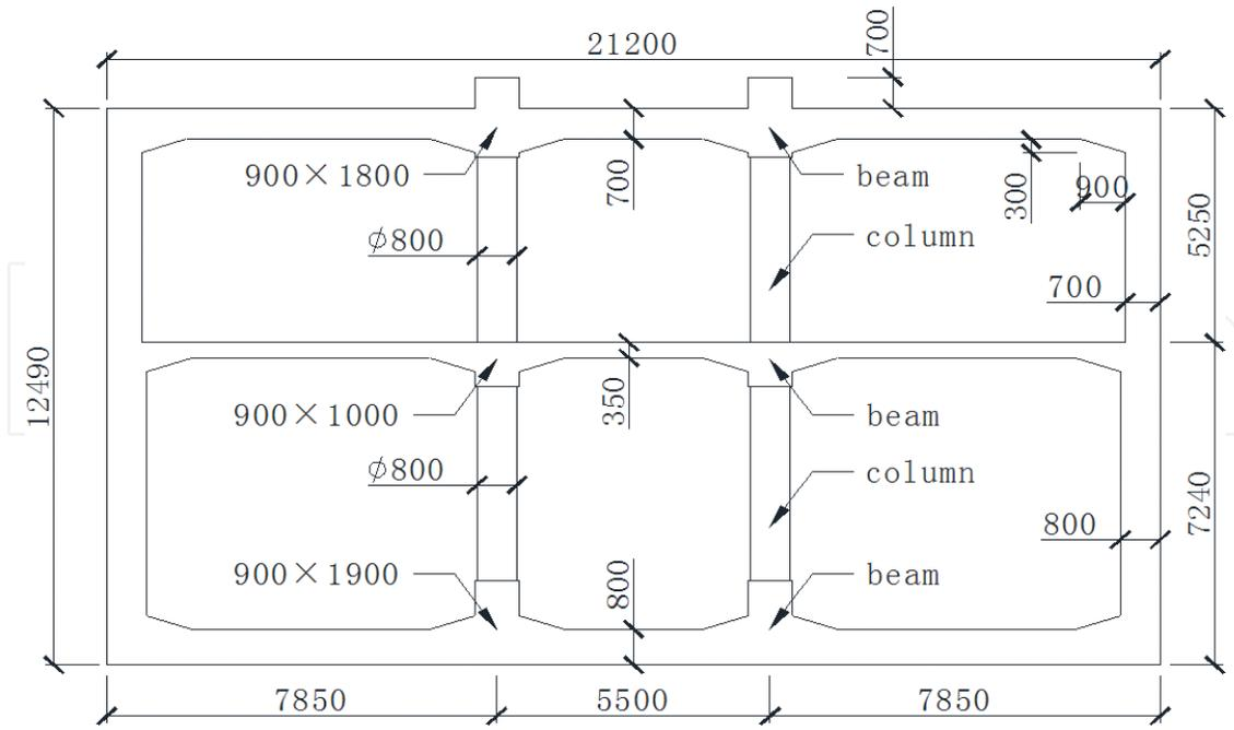
Figure 2. Cross-section of underground station (unit: Mm).
