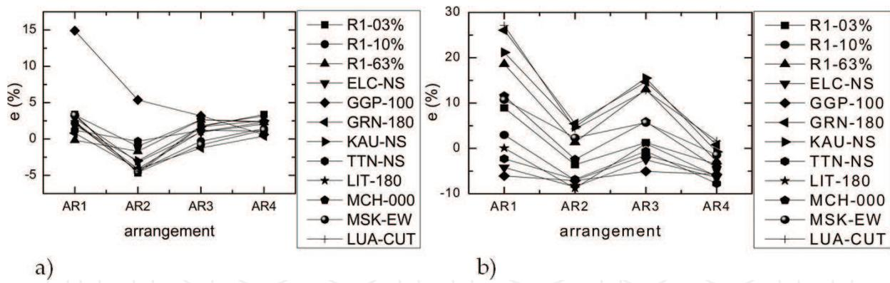
**Figure 18.** Interaction between surface structure and underground structure in terms of influence coefficient  $e$  for different arrangements under S waves producing motions along lateral axis ( $d = 0.5$ ), a) the impact on surface structure, b) the impact on underground structure.
