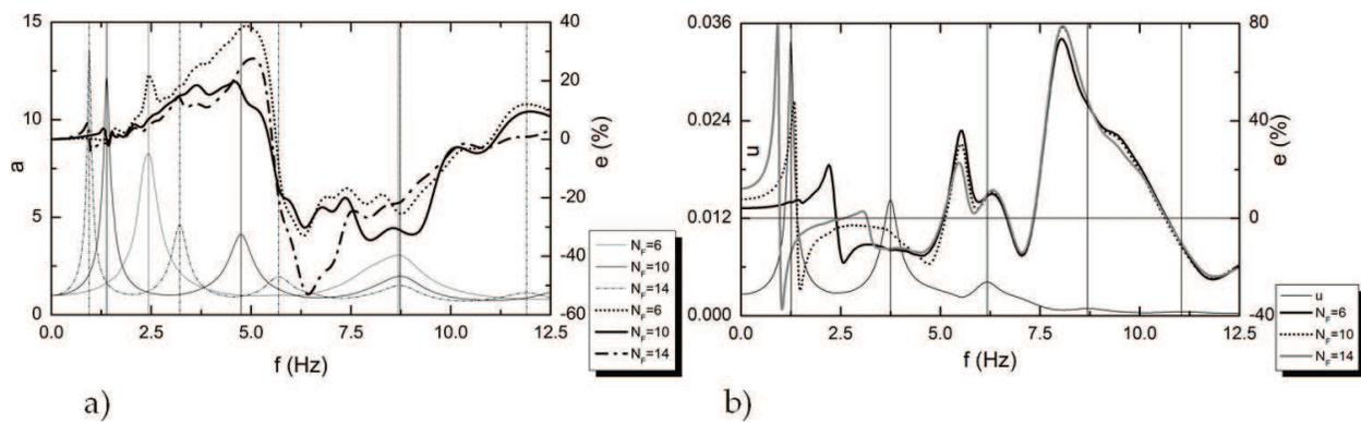
**Figure 13.** Interaction between surface structure and underground structure, arranged according to AR1, in terms of harmonic response spectra and influence coefficient  $e$  for different number of storey of surface structure under S waves producing motions on the Y axis ( $d = 0.5$ ), a) the impact on surface structure, b) the impact on underground structure.
