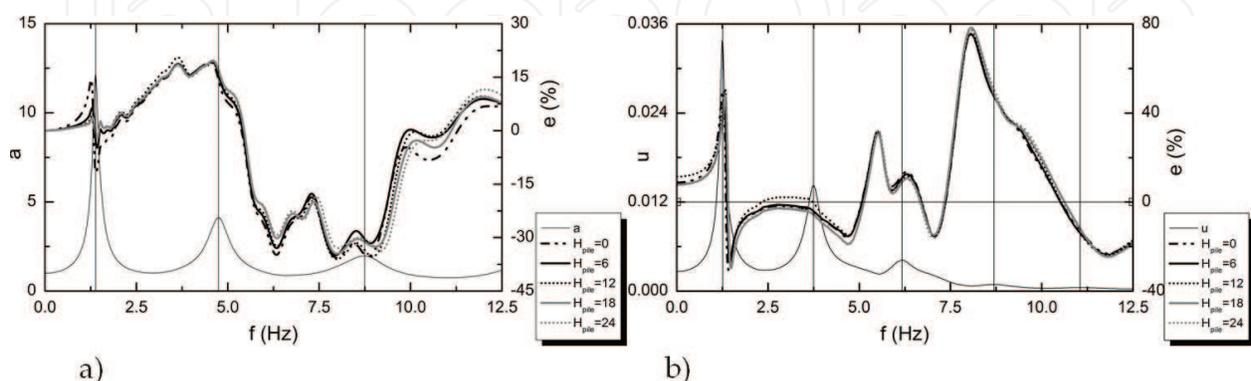
**Figure 10.** Interaction between surface structure and underground structure, arranged according to AR1, in terms of harmonic response spectra and influence coefficient  $e$  for different length of pile of surface structure under S waves producing motions on the Y axis ( $d = 0.5$ ), a) the impact on surface structure, b) the impact on underground structure.
