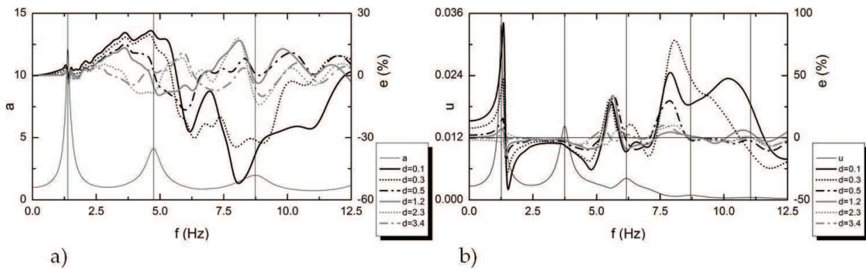
**Figure 7.** Interaction between surface structure and underground structure, arranged according to AR1, in terms of harmonic response spectra and influence coefficient  $e$  for different distances between structures under S waves producing motions on the Y axis, a) the impact on surface structure, b) the impact on underground structure.
