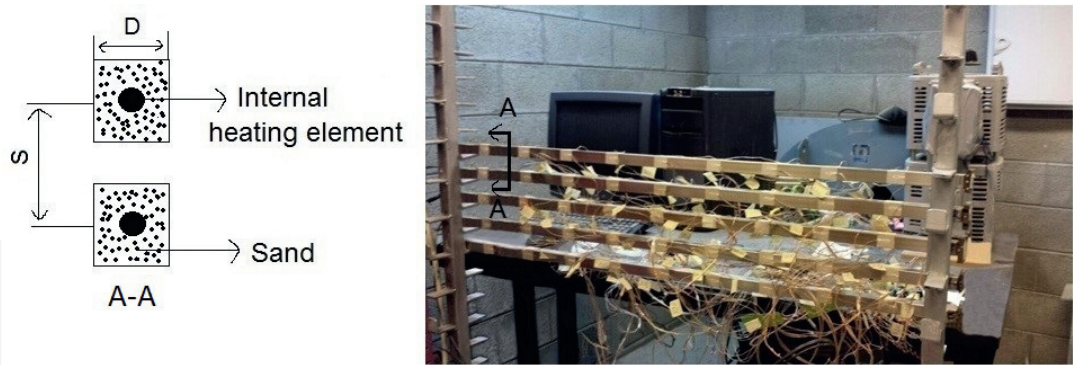
Figure 1. Setup used to hold the arrays of square cylinders and cross sections at A-A showing the center-to-center distance S and the side length D of the square cylinders.
