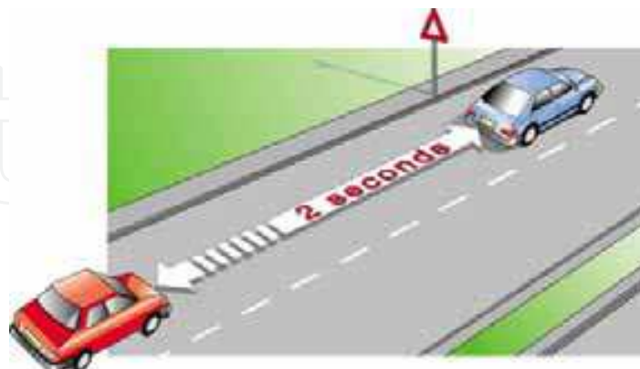
Fig. 8. Safe Distance decision by applying two seconds rule
