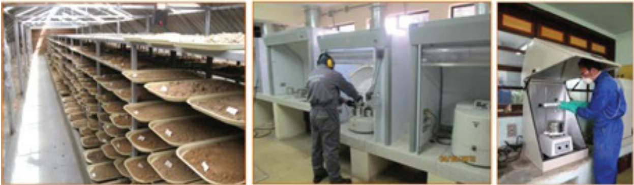
Figure 16. Sample preparation process: (a) drying (b) grinding and (c) screening.
