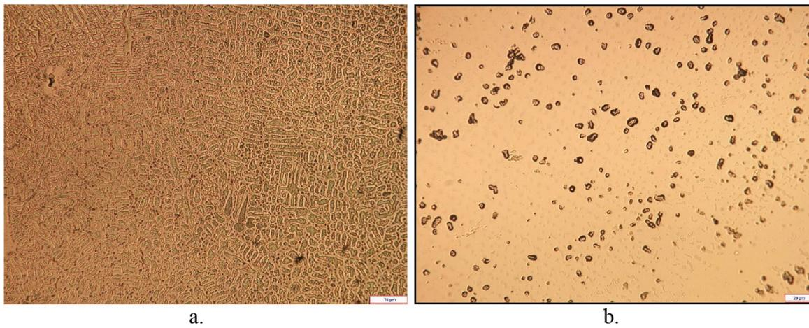
**Figure 25.** Wironit extra-hard (Bego) sample. (a) Welded on both sides, with nonuniform dendritic structure. (b) With thermal treatment, with nonuniform fine dendritic structure and carbide inclusions.
