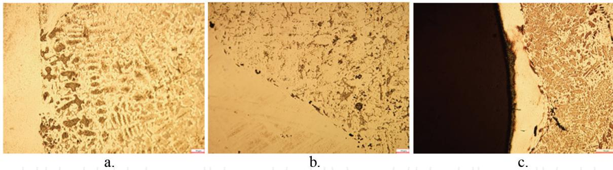
**Figure 35.** Microscopic aspect of the welded CoCrMoZrTi alloy using different parameter values: (a) first set, (b) second set, (c) third set.
