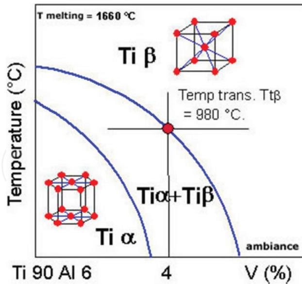
Figure 9. Schematic pseudo-binary phase diagram of TA6V4 alloy.
