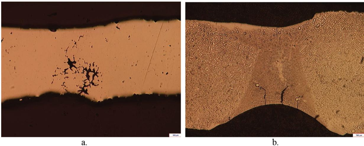
**Figure 24.** (a) Nonuniform dendritic structure with interdendritic cracks and microporosities. (b) Microstructural aspect of the welding cord in case of “C” alloy (Vaskut Kohászati Kft), with cracks due to laser exposure, spreading from surface to center.
