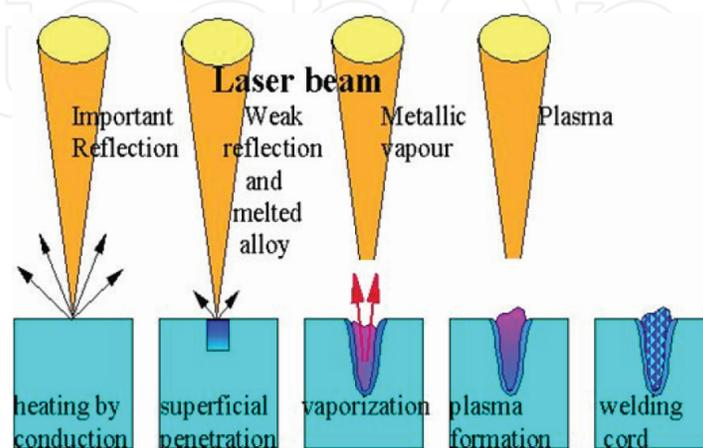
**Figure 5.** Stages of the welding cord formation.
