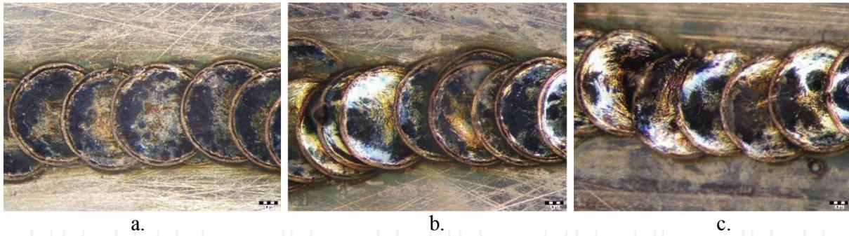
**Figure 32.** Macroscopic aspect of the welded CoCrMoZrTi alloy using different parameter values: (a) first set, (b) second set, (c) third set.
