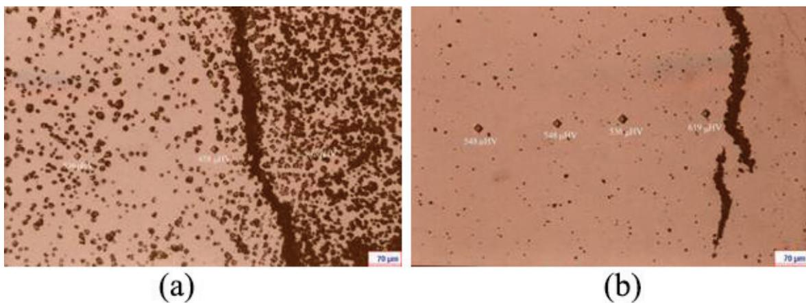
**Figure 27.** Microstructural aspect of Wironit extra-hard (Bego) laser welded samples. (a) TAA microhardness values lower up to 15%. (b) Samples with heat treatment, TAA microhardness values higher up to 16%.
