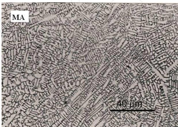
Figure 14. MA area (metallography).
