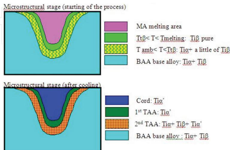
Figure 10. Schematic description of the cord during welding.
