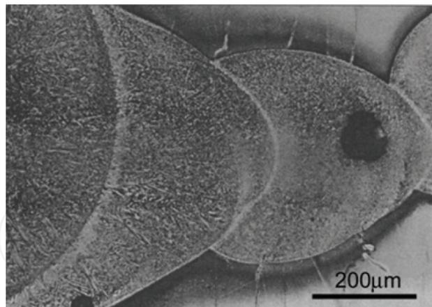
Figure 12. Welded area (SEM).
