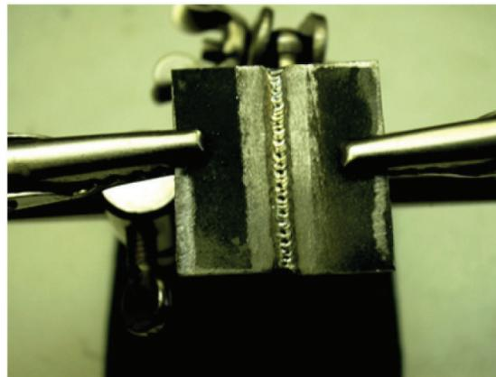
**Figure 7.** Micro pulse welded piece.
