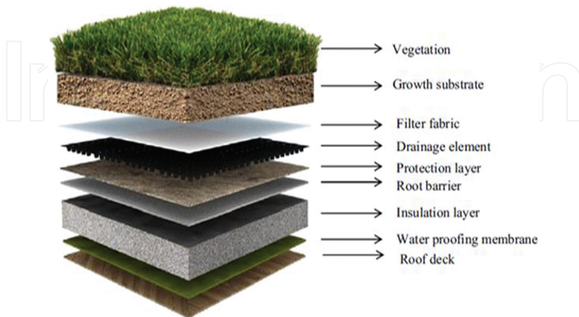
Figure 10. Schematics of different green roof components [58].
