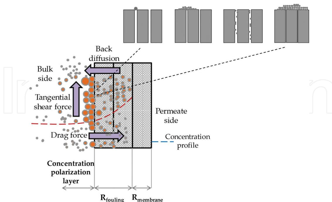
**Figure 1.** Concentration polarization and membrane fouling mechanisms during membrane filtration: from left to right, (i) pore sealing or complete pore blocking, (ii) intermediate pore blocking, (iii) standard blocking or pore filling/constriction, and (iv) cake or gel layer (adapted from Ochando-Pulido and Martínez-Férez [29]).
