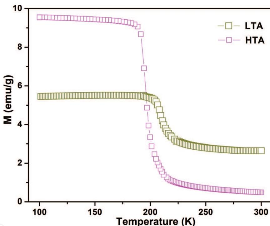
**Figure 2.** Temperature dependence of magnetization of  $\text{La}_{0.7}\text{Pr}_{0.3}\text{Fe}_{11.4}\text{Si}_{1.6}$  for LTA and HTA.
