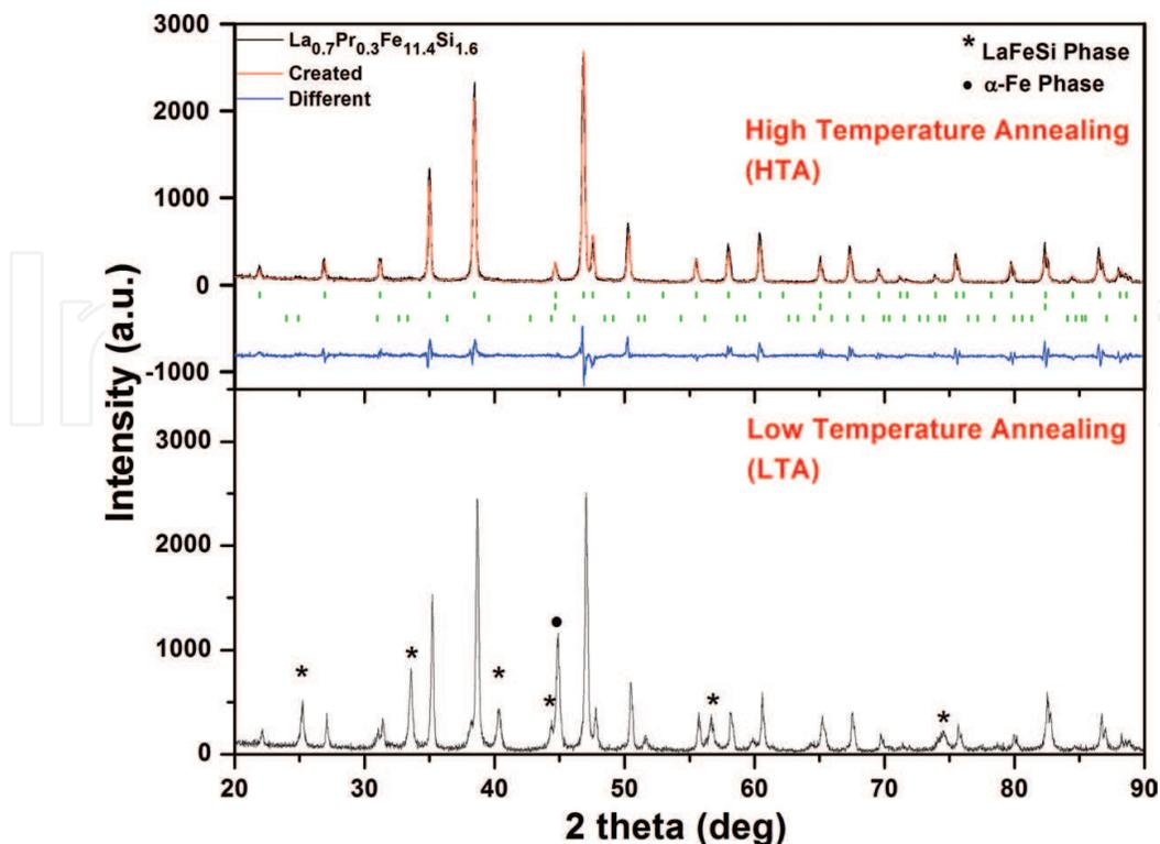
**Figure 1.** Room temperature X-ray diffraction patterns of La<sub>0.7</sub>Pr<sub>0.3</sub>Fe<sub>11.4</sub>Si<sub>1.6</sub> produced by the HTA and LTA processes.
