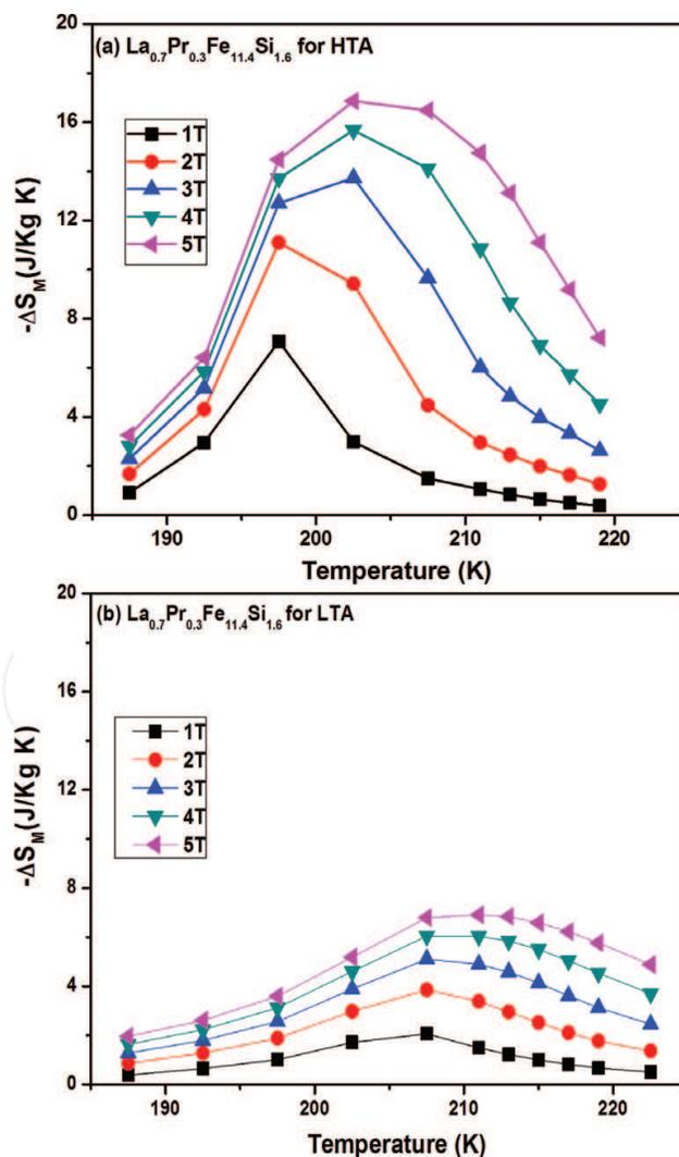
Figure 4. Magnetic entropy change,  $-\Delta S_m$ , for a 0-5 T change in field of  $\text{La}_{0.7}\text{Pr}_{0.3}\text{Fe}_{11.4}\text{Si}_{1.6}$  for (a) HTA and (b) LTA compounds as a function of temperature.
