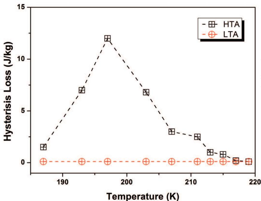
**Figure 3.** Comparison of the magnetic hysteresis losses for  $\text{La}_{0.7}\text{Pr}_{0.3}\text{Fe}_{11.4}\text{Si}_{1.6}$  produced by the HTA and LTA process under magnetic fields over the ranges  $B = 0\text{--}5$  T.
