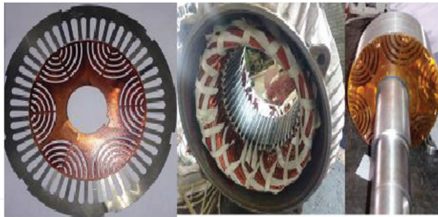
Figure 12. Fabrication details of 8-6-4 BDFRM.
