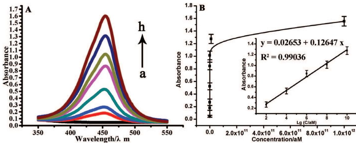
Figure 5. (A) Absorption spectrum response of the assay with different target DNA (0, 0.01 fM, 0.1 fM, 10 fM, 1 pM, 100 pM, 10 nM and 1  $\mu$ M). (B) Calibration curve of the DNA assay with different concentrations of target DNA. Standard deviation was represented as error bars,  $n = 3$ .
