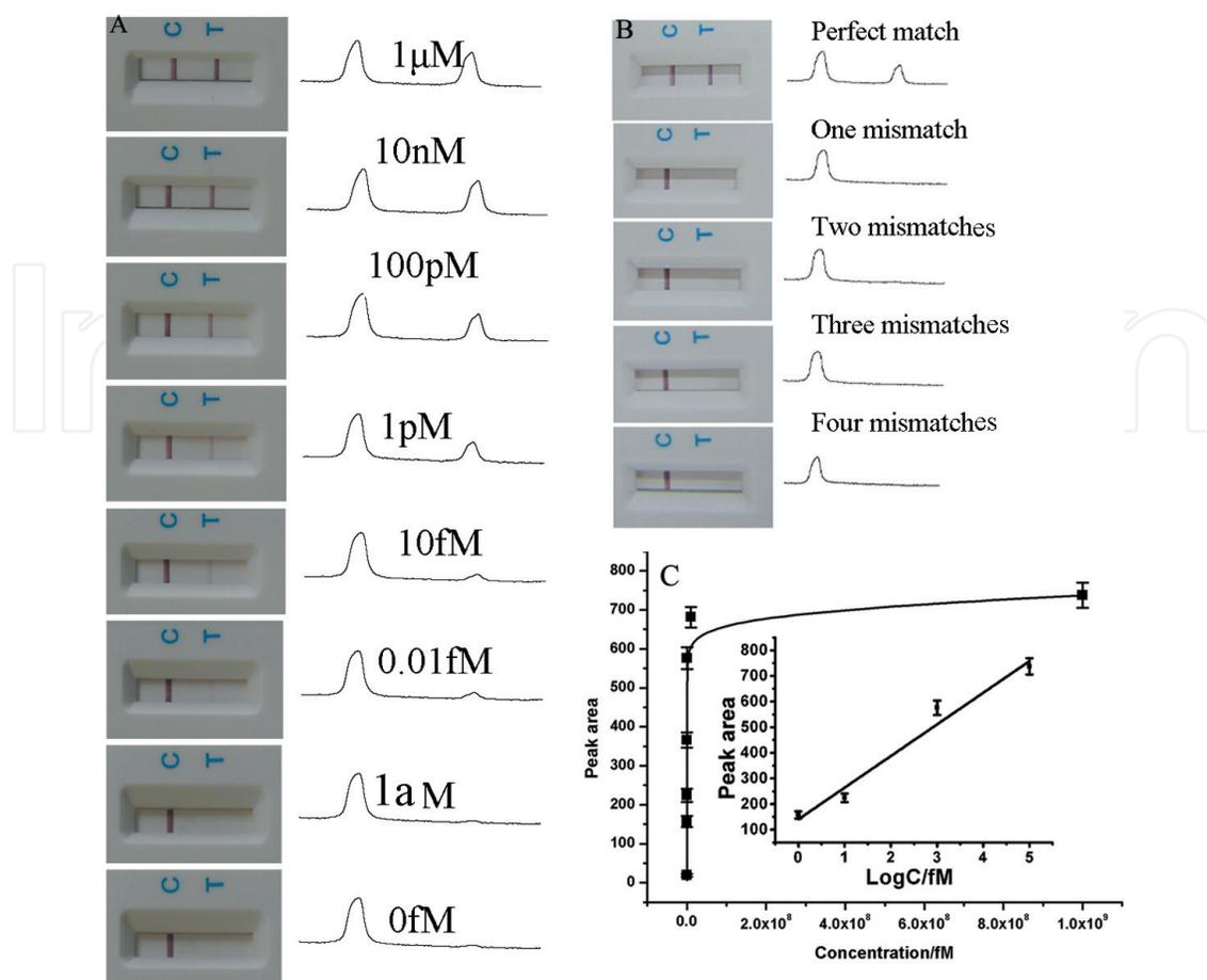
**Figure 3.** (A) Typical photographic images (left) and corresponding intensities (right) of an LFNAB in the presence of various concentrations of synthetic target DNA and the negative control. (B) Photographic images (left) and corresponding intensities (right) of the LFNAB tested with target DNA and target DNA including one or more mismatched bases. (C) Calibration curve of an LFNAB with various concentrations of target DNA. The error bars represent the standard deviations,  $n = 3$ .
