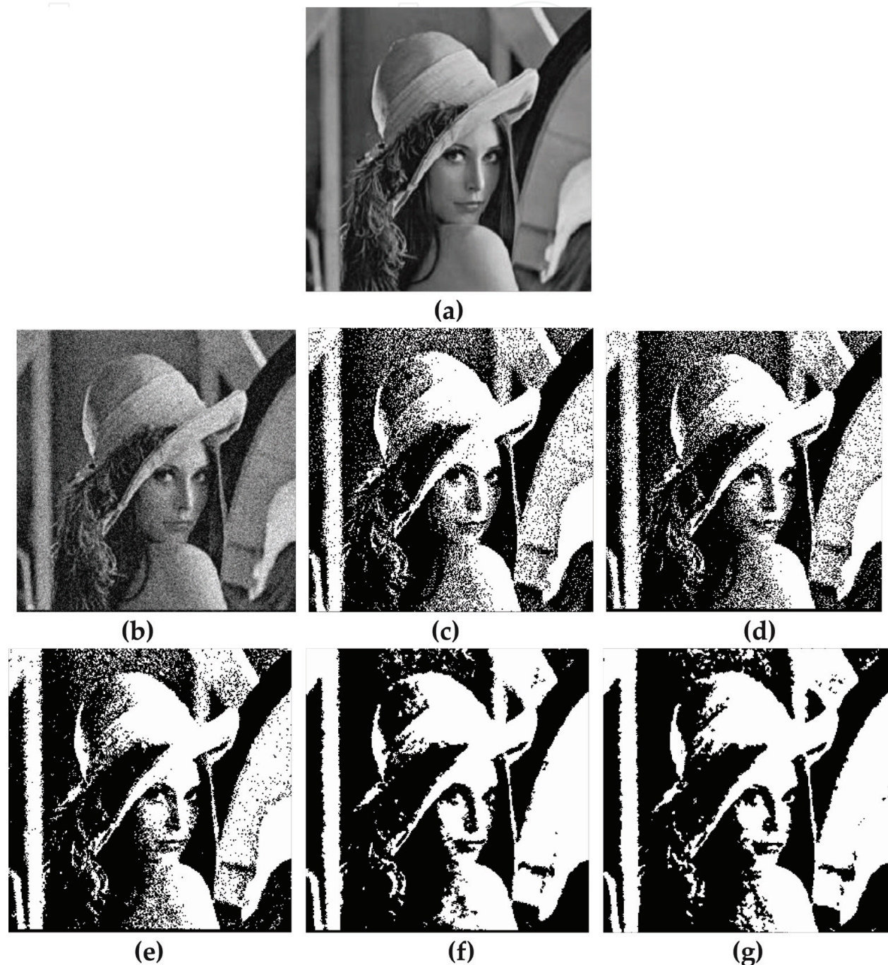
Figure 5. Segmentation of Lena image: (a), noise-free image; (b), the image in (a) plus WGN noise with zero-mean and 0.05 variance. It is obvious that the images in (f) and (g) have lesser number of misclassified pixels. The clustering validation coefficients summarized in Table 2 which shows that the LMKLFCM and the LDMKLFCM algorithms provide the superior V_{PC} and V_{PE} .
