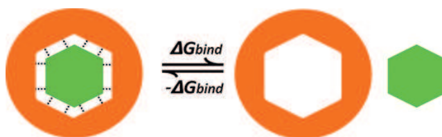
Figure 2. Schematic representations of a reversible non-covalent association/dissociation process of a guest molecule (green) and a host (orange) molecule, possessing a certain binding energy difference ( \Delta G_{\text{bind}} ) between the associated and dissociated states.
