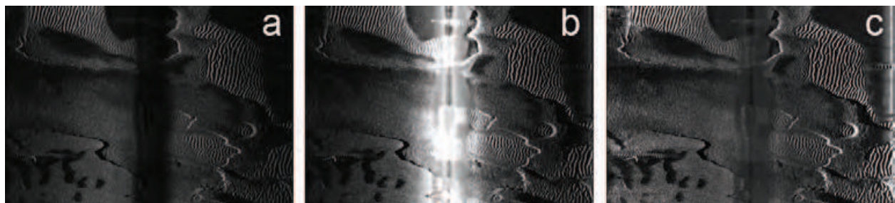
Fig. 8. The recovered beam-profile projection can be used to level the intensities of the ground-range version of the sonar image. (a) The original TVG-corrected sonar image in ground-range coordinates after proper projection using the recovered elevation map. (b) How would the image look if the beam-profile of the sonar was isotropic (had the same intensity on all grazing angles). (c) Ground-range image with a modified beam-profile that ensures an even illumination at all average incidence angles; this is the texture map that has been used on Figures 6(c) and 7.
