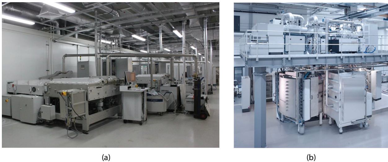
Figure 9. Laboratory installation (a) and industrial PECVD system (b).
