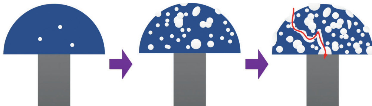
Figure 12. Nucleation, growth and saturation stage diagram of PCM cell in the SET process.
