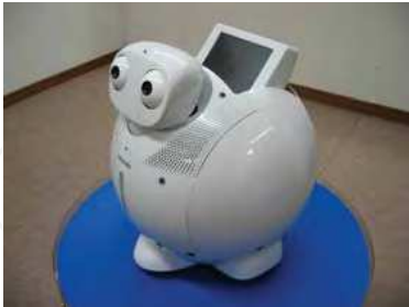
Fig. 6. Sharp ear robot ApriAlpha™ V3.
