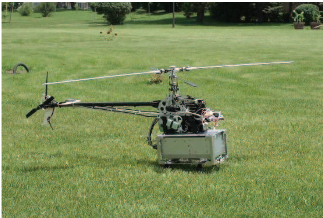
Figure 4. Implemented rotorcraft UAV
