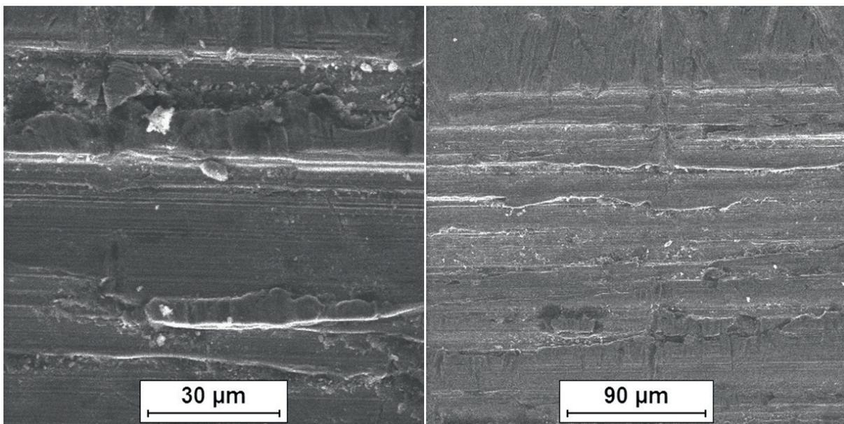
**Figure 20.** Surface of the roller axle of the control unit made of intermetallic alloy Fe<sub>40</sub>Al<sub>5</sub>Cr<sub>0.2</sub>TiB.
