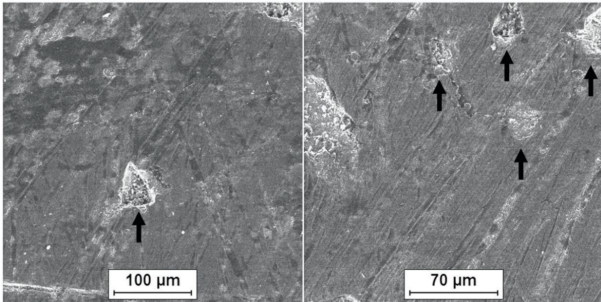
**Figure 19.** Surface view of the roll axis control system made Fe<sub>40</sub>Al<sub>5</sub>Cr<sub>0.2</sub>TiB intermetallic alloy. Visible metallurgical defects in the form of shrinkage porosity.
