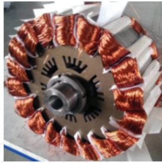
Figure 12. Stator windings of OR-SRM at manufacturing stage.
