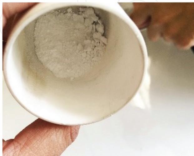
**Figure 2.** The BCABS-1ZrO<sub>2</sub> was prepared after drying in the over at  $150^\circ C$  for 4 h.
