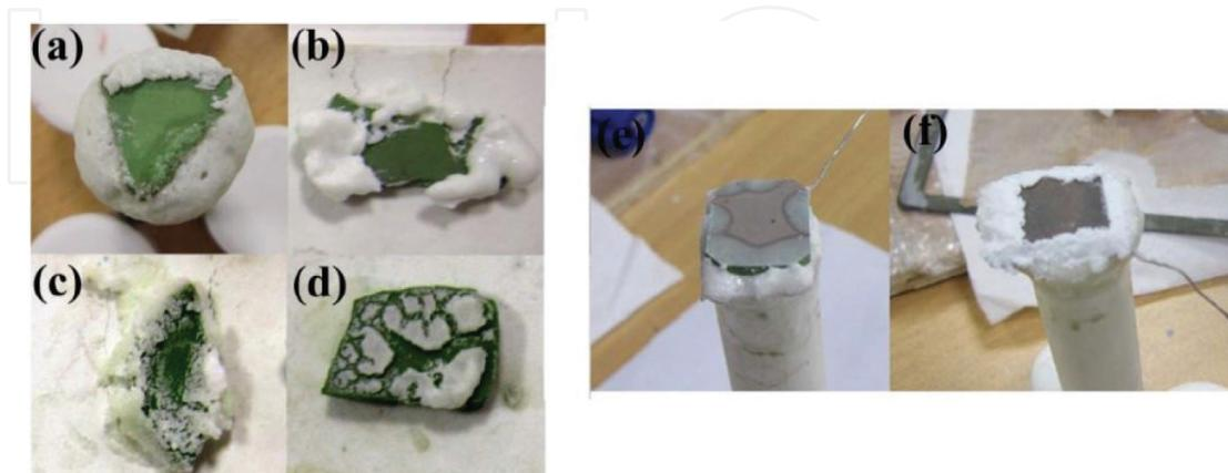
**Figure 4.** Comparison of the chemical reaction between glass ceramic sealant and solid oxide fuel cell: (a) BCABS, (b) BCABS-1 $ZrO_2$ , (c) BCABS-2 $ZrO_2$ , and (d) BCABS-3 $ZrO_2$ . Picture exhibits the comparison of glass ceramic sealants: (e) BCABS and (f) BCABS-1 $ZrO_2$  [9].
