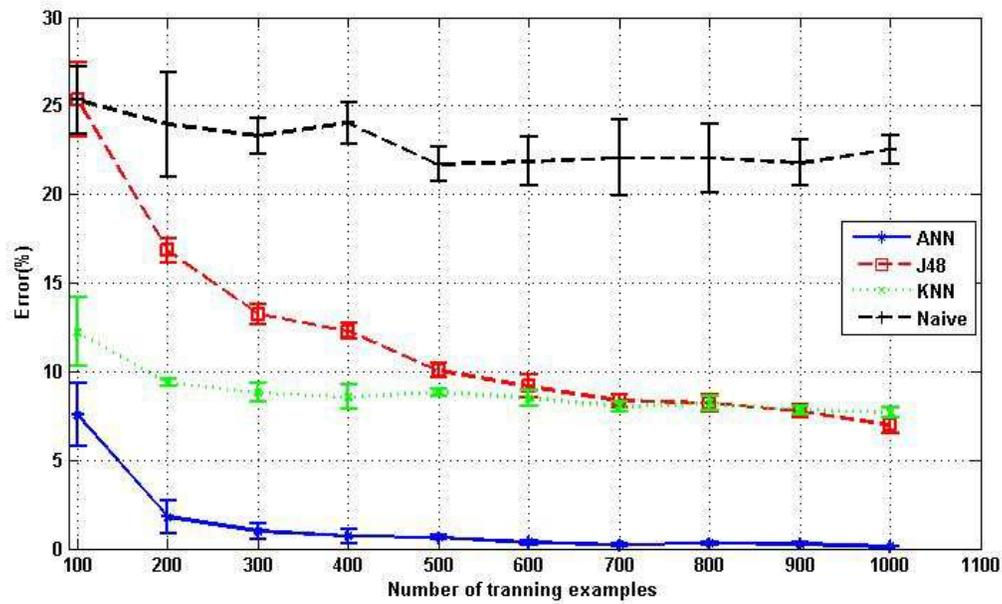
Fig. 11. Sample complexity for frame-based classification (the error is  $E_f$ ) with  $L = S = 9$ . The figure shows the average and standard deviation. It can be seen that approximately  $M = 700$  examples suffices to train the classifiers.
