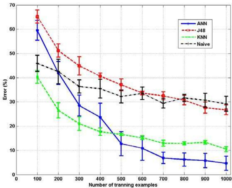
Fig. 12. Sample-complexity for one-frame-based classification with  $L = S = 9$  (error  $E_o$ ). The figure shows the mean and standard deviation. It can be seen that the error has a more erratic behavior than in Figure 11.
