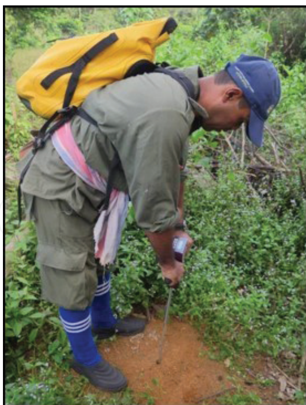
Figure 4. Measuring of soil compaction through penetrometer.
