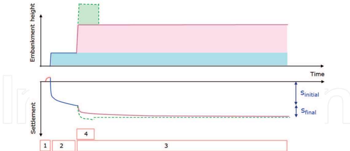
Figure 7. Phases of settlement in mass stabilized layer and settlement time diagram [45].
