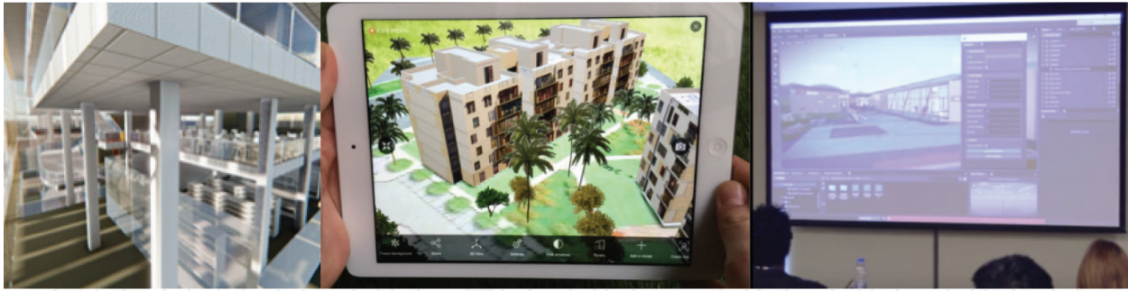
Figure 1. Virtual reality tour inside and outside a BIM model and supporting a collaborative meeting.
