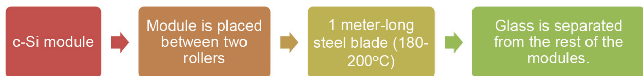
Figure 9. Summary of “hot knife” recycling process for PV modules [46].
