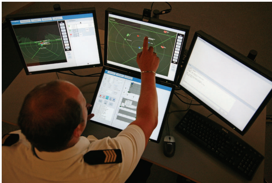
Figure 5. The Basic-T functions as a test bed for the design and evaluation of future combat management workstations
