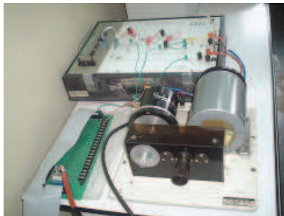
Figure 2. Actual DC motor experiment device
