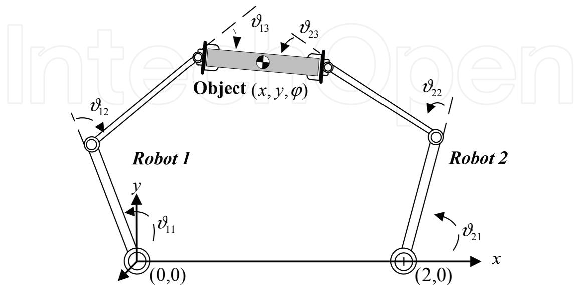
Figure 3. A two-link planer constrained robot manipulator
