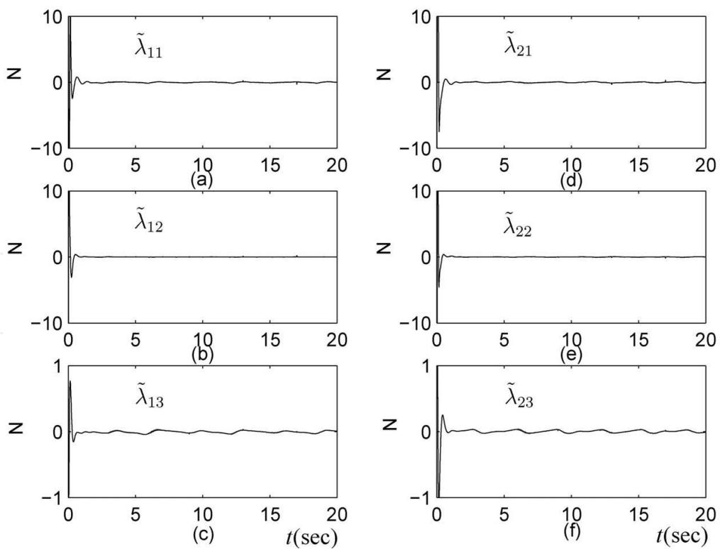
Figure 6. (a-c) Internal force tracking errors for Robot 1; and (d-f) internal force tracking errors for Robot 2
