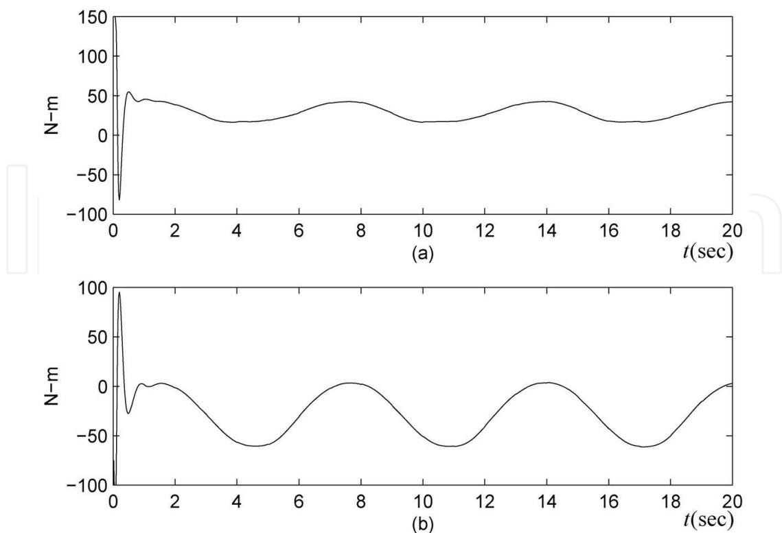
Figure 7. (a) Control input for the second joint of Robot 1; and (b) control input for the second joint of Robot 2
