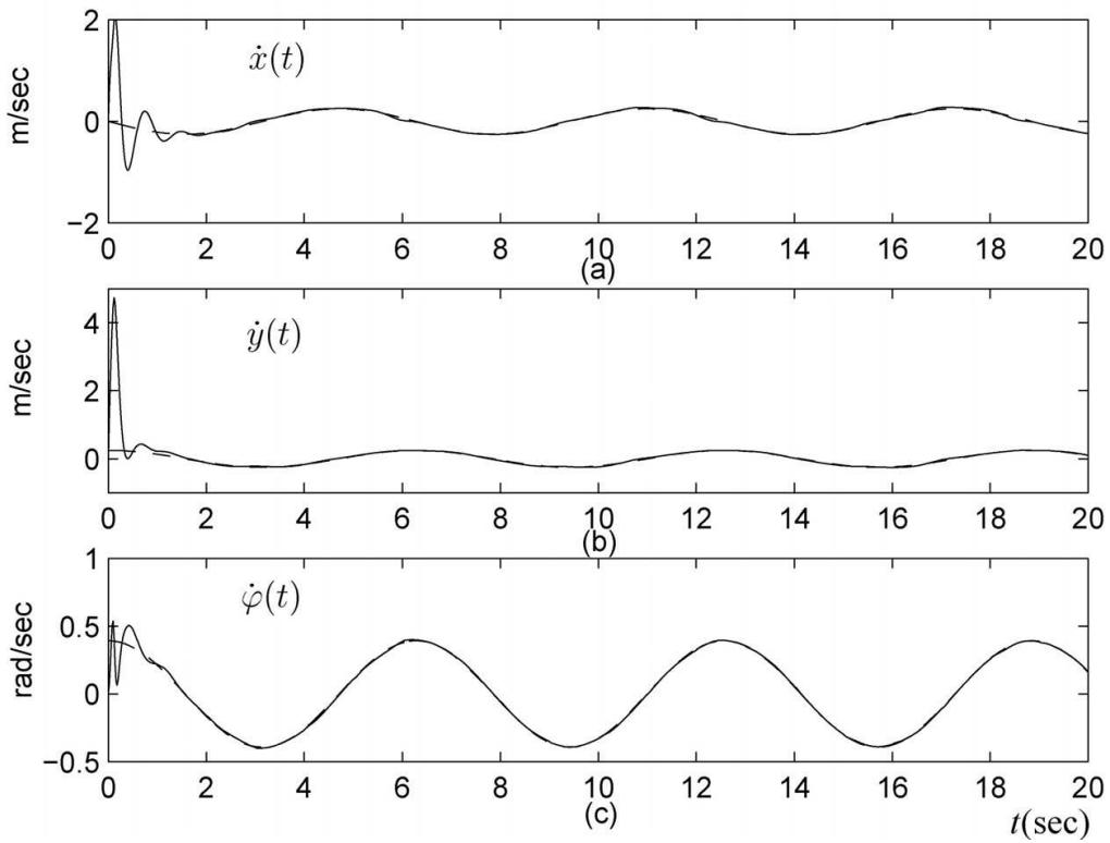
Figure 5. The velocity tracking results of the held object. (— object, - - reference)
